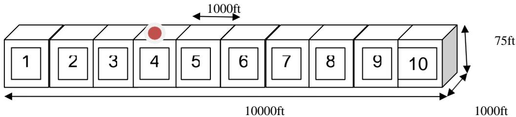
Figure 3.1: Reservoir grid blocks
