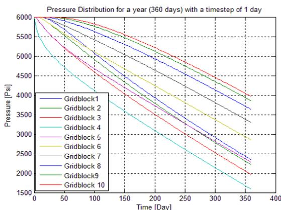
Figure 4.1: Pressure distribution for a year with a time step of 1 day.
