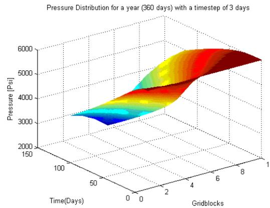
Figure 4.6: 3-D view of pressure distribution for a year with a time step of 3 days
