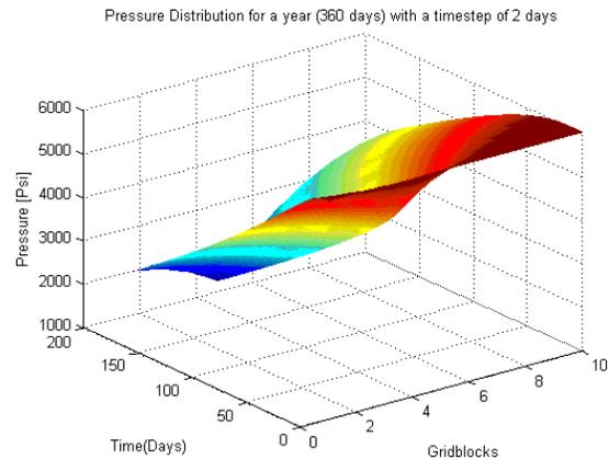
Figure 4.4: 3-D view of pressure distribution for a year with a time step of 2 days
