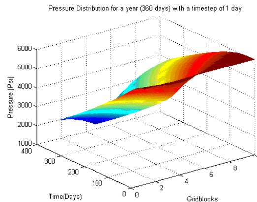
Figure 4.2. 3-D view of pressure distribution for a year with a time step of 1 day
