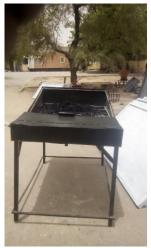
FIG. 1: A picture of wick tilted solar still
