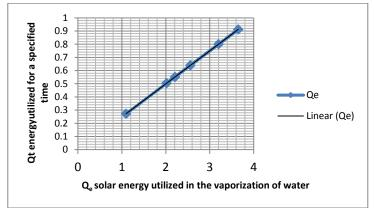
Figure2 : The relation between the energy utilized in the vaporization of water over the latent heat of vaporization and the energy absorbed for a specified time falling on the system Table 1:The various values of the  $Q_t$  and  $Q_e$
