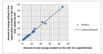
Figure 3 above: shows the relation amount of energy utilized in the vaporization of water and amount of solar energy incident on the still
