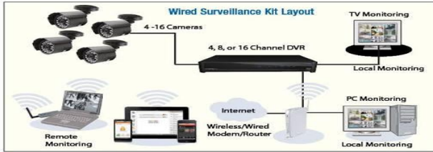
Fig.1 Schematic diagram for IP surveillance system (Image courtesy en.wikipedia.org)
