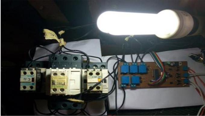
Fig.7: MCU interfaced with contactors for testing
