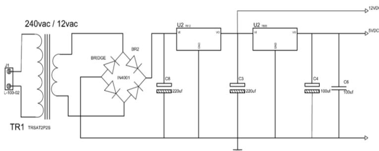
Fig 2: Power supply diagram
