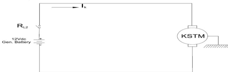
Fig.4: A section showing how the generator kick starter motor (KSTM) was interfaced with the MCU.
