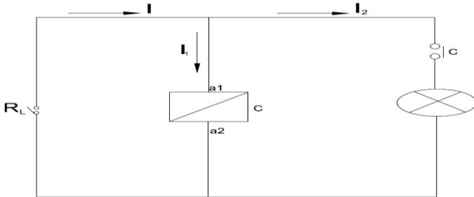
Fig. 3: Diagram showing how each contactor coil is interfaced by the MCU via low voltage relays
