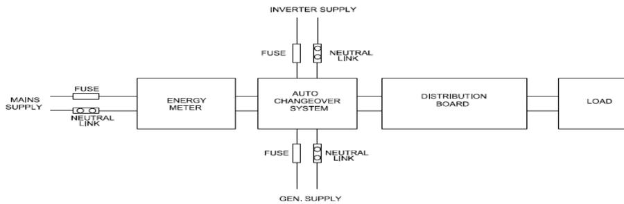
Fig. 10: Block diagram showing installation of system
