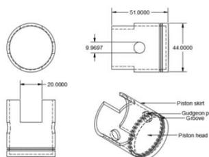
Figure 4: Third Angle Orthographic Projection
