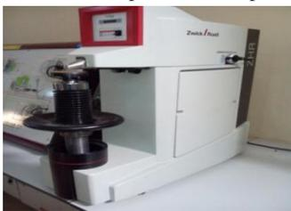
Figure 1: Rockwell hardness machine
