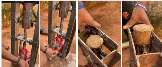
Figure 2: The compaction process
