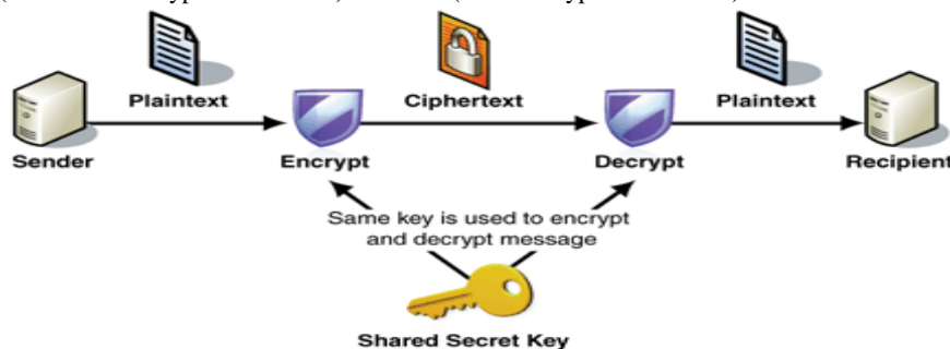
Fig1: Symmetric Key Encryption
