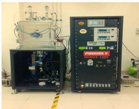
Figure 1 R. F Magnetron sputtering vacuum chamber and control panel.
