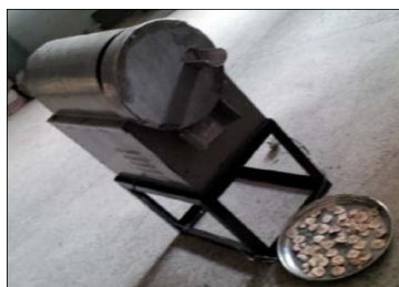
Plate1: Motorized Plantain slicing machine (Adesina et al., 2015)
