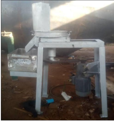
Plate.2: Picture of the constructed damage efficient Plantain Slicing Machine
