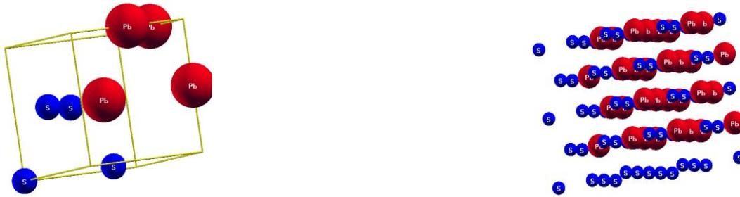
Figure 1: RocksaltPbS crystal structure. The blue atoms are the sulphur atoms while the red atoms are the Lead atoms. On the left (a) is the conventional unit cell while on the right (b) is the 3x3x3 repeated cell to show the full arrangement of the atom in a bulk like case.
