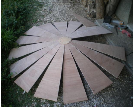
PLATE 1: Dividing plywood for construction of parabolic dish into 15 equal parts
