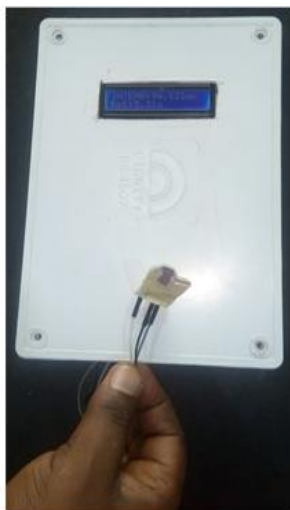
Figure 7: The complete assembly of the locally developed lux-meter
