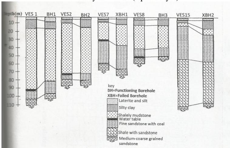
Figure 10: Correlation of borehole (BH) log with subsurface geoelectric sections of VES 1, 2, 7, 8, and 15
