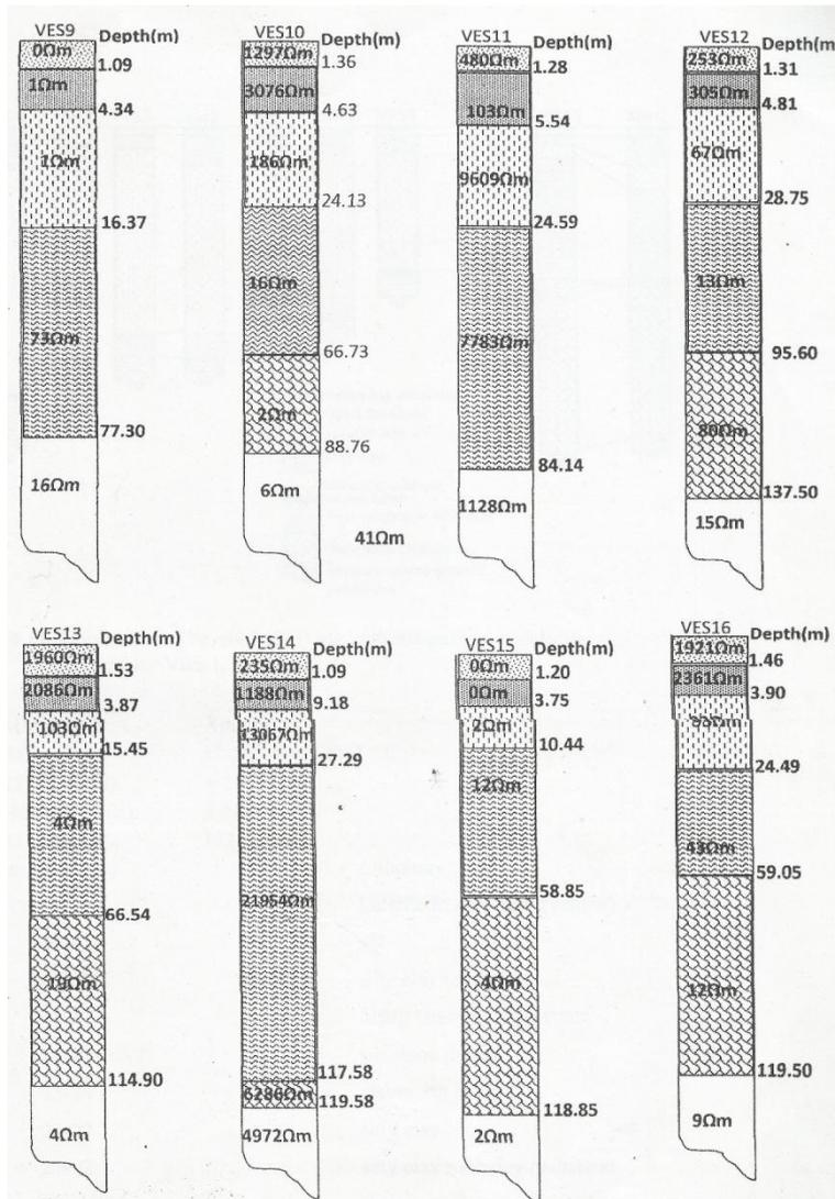
Figure 9: The VES layers and lithology for VES 9-16 deduced from computer interactive model
