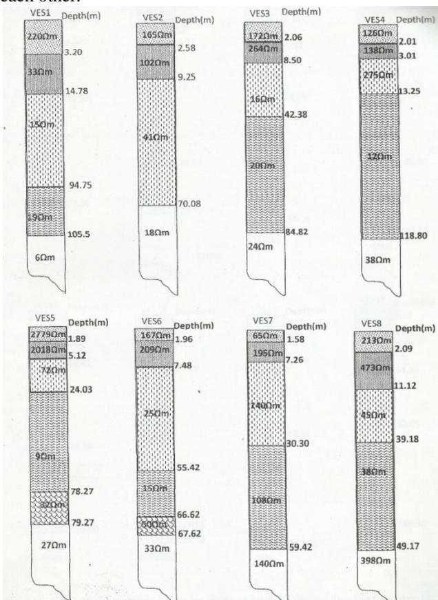
Figure 8: The VES layers and lithology for VES 1-8 deduced from computer interactive model
