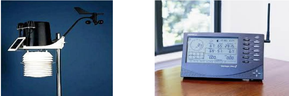
Fig. 1: The experimental set-up (a) the integrated sensor suite and (b) the console
