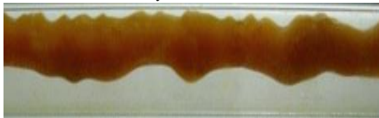
Figure 4.7: Stratified wavy flow, experimental result(Anand, et al., 2013, p. 77)
