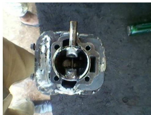
Fig. 7: Cast Engine Block after Machining and Cleaning
