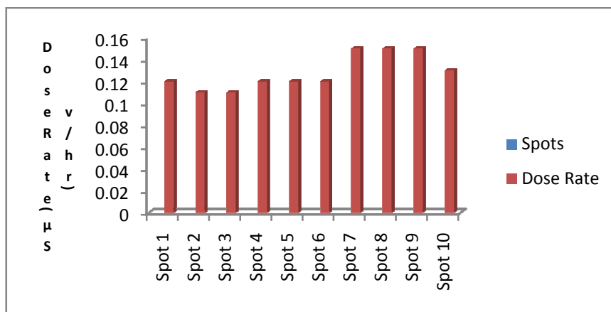
Fig 3: Pictorial Representation of In-situ Dose Rate( \mu\text{Sv}/\text{hr} ) at Ijebu – Ode Dump Site
