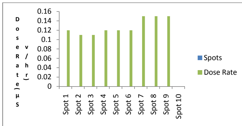
Fig 2: Pictorial Representation of In-situ Dose Rate( \mu\text{Sv}/\text{hr} ) at Ijebu – Igbo Dump Site
