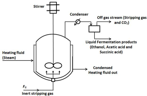
Figure 1: Schematic diagram of batch fermentation process coupled with gas stripping
