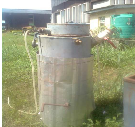
Fig. 2: Locally made biogas digester Ref: [11].
