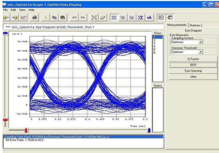
**Fig 12:** Screenshot of eye diagram for 1<sup>st</sup> run
