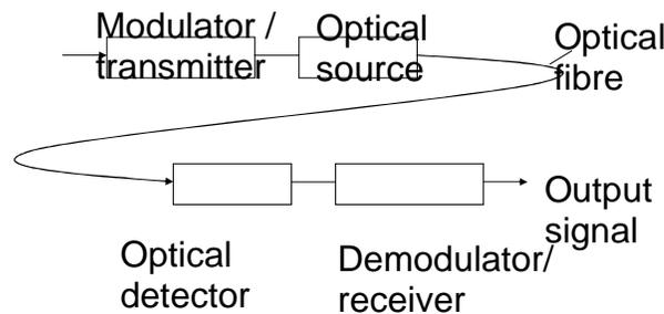
**Fig 1:** The Basic fibre Optics Transmission System
