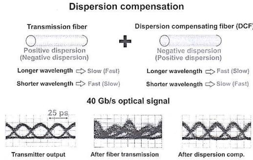
**Fig 6:**Dispersion through fibers of 50Km length at 40 Gb/s Bandwidth
