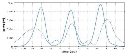
**Fig 9:** Pulse distortion after 10 km (solid curve) and 50 km (dashed curve) of a dispersion-shifted fibre, when only second-order dispersion is compensated.
