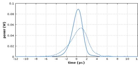
**Fig 8:** Distortion of a triple pulse after 10 km (solid curve) and 50 km (dashed curve) of a dispersion shifted fibre, when only second-order dispersion is compensated.
