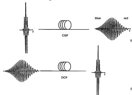
**Fig 5:**(a) Unchirped Pulse (b) Compressed Chirped Pulse
