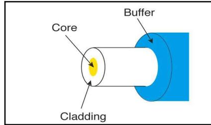
**Fig 2: Structure of Optical Fiber**
