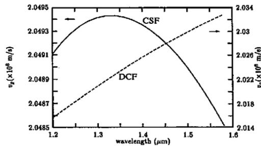
**Fig4:** Graph of Pulse through Dispersion Compensation Fiber and Conventional Single Mode Fiber
