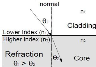
**Fig 3: Refraction of light**
