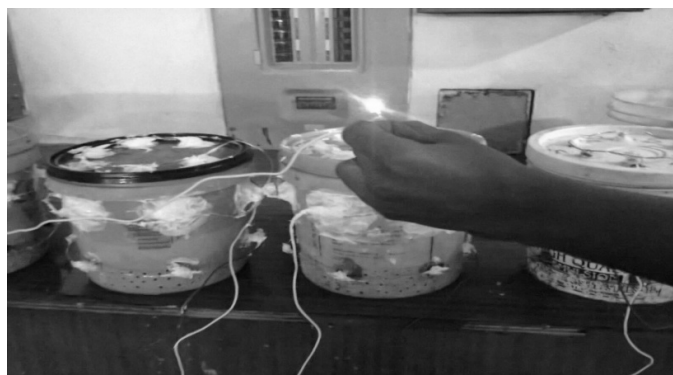
Fig. 9: Five (5) Metal/Air Fuel Cells used to Power a 4V Bulb
