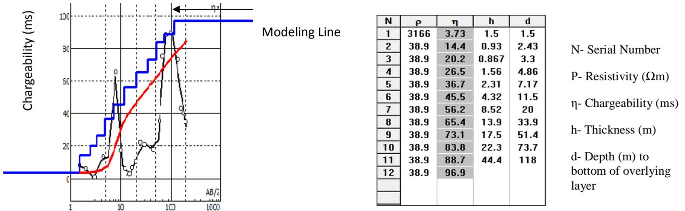
Figure 4: IP Curve and corresponding model parameters Table for VES 1
