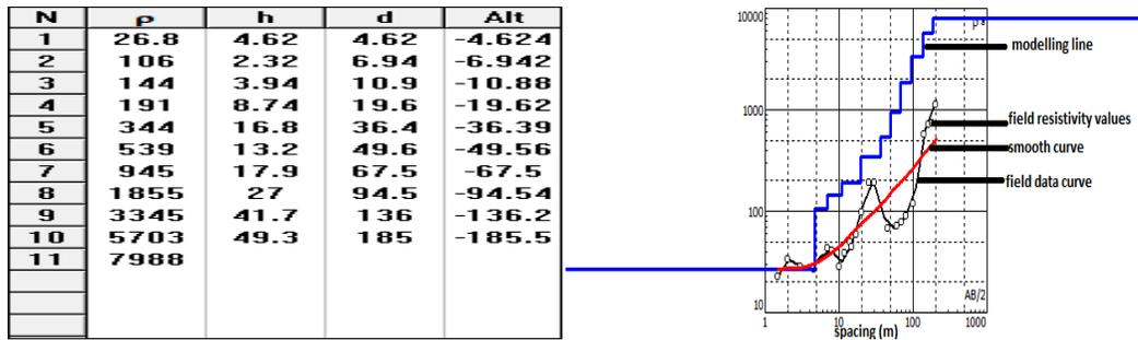
Figure 5: Resistivity Curve and corresponding model Parameters Table for VES 1
