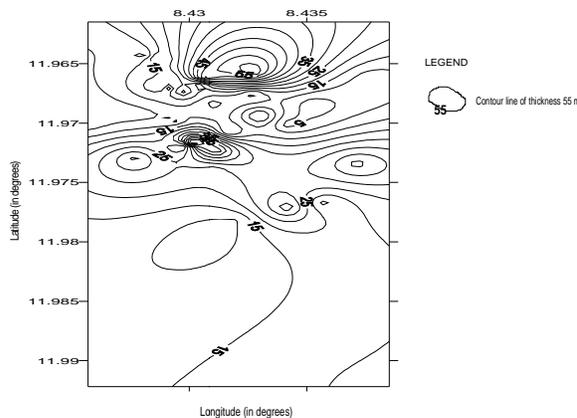
Figure 7: Aquifer Thickness Map contoured at 5m interval
