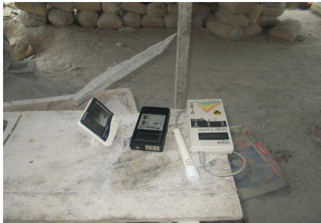
Fig. 1: Setup of the apparatus for measurement of background gamma radiation, temperature and humidity
