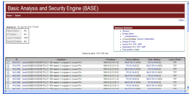
Figure 7: 1 to 48 of 290 alerts triggered for signature based detection using IDEVAL DARPA dataset.
