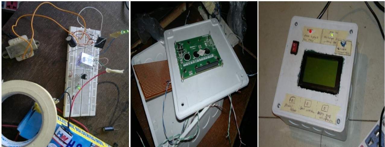
Fig.8: (a) Power supply on Vero board. (b) Housing the Oscilloscope. (C) The assembled digital oscilloscope.
