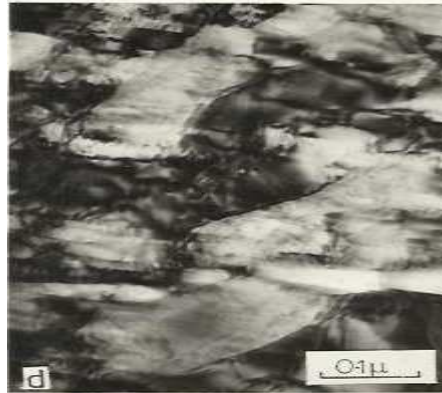
Plate 8: U50A deformed 20% at -196°C and annealed at 700°C: Bright Field (BF) image of untransformed \gamma revealing extensive recovery and persistent deformation-induced banded morphology
