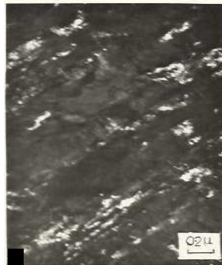
Plate 5: High Resolution Dark Field (HRDF): U50D deformed 80% at -196°C, showing thin inter-lath untransformed austenite reversed \gamma
