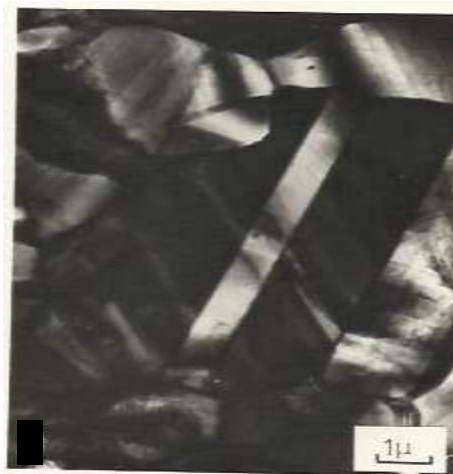
Plate 7: U50D deformed 20% at -196°C followed by 3 minutes at 900°C. Recrystallized \gamma has developed annealing twins
