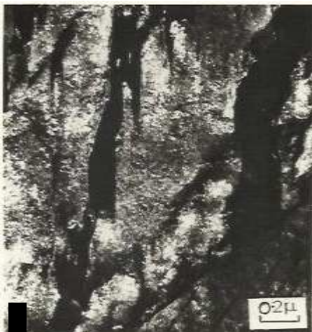
Plate 6: High Resolution Dark Field (HRDF): U50D deformed 20% at -196°C. Dark regions is untransformed \gamma . The martensite laths appear to exhibit cell-structural appearance of dislocation.
