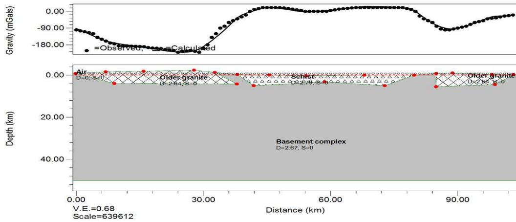
Figure 4.2: Two and half dimensional model of residual anomaly along profile BB'
