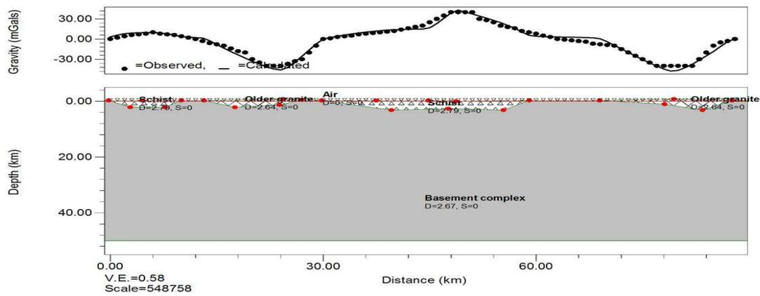
Figure 4.3: Two and half dimensional model of residual anomaly along profile CC'
