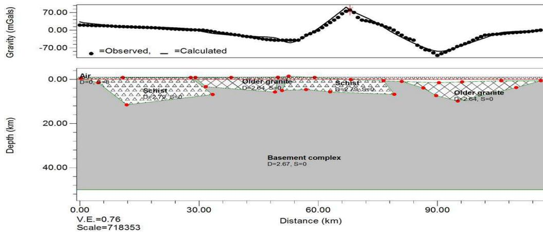
Figure 4.4: Two and half dimensional model of residual anomaly along profile DD'
