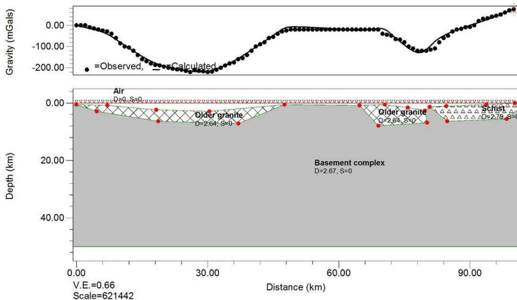
Figure 4.1: Two and half dimensional model of residual anomaly along profile AA'
