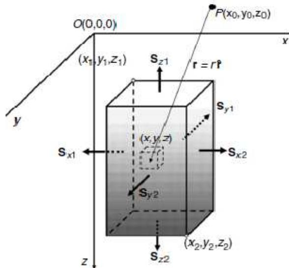
**Figure 2:** Drawing demonstrating the gravity anomaly at an observation point  $P(x_0, y_0, z_0)$  resulting from a mass element at source point  $P(x, y, z)$ .
