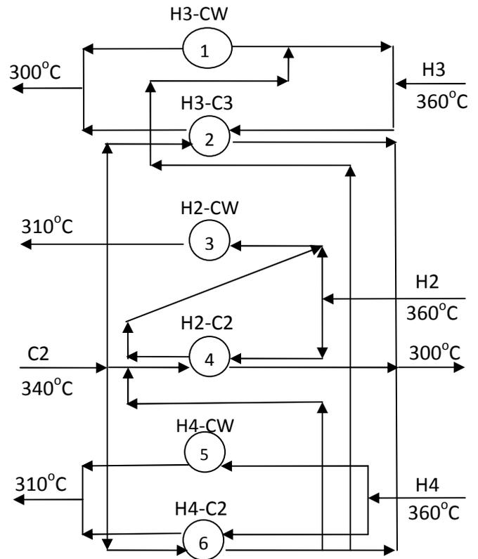
Figure 5: Heat exchanger superstructure for stream matches above the pinch point
