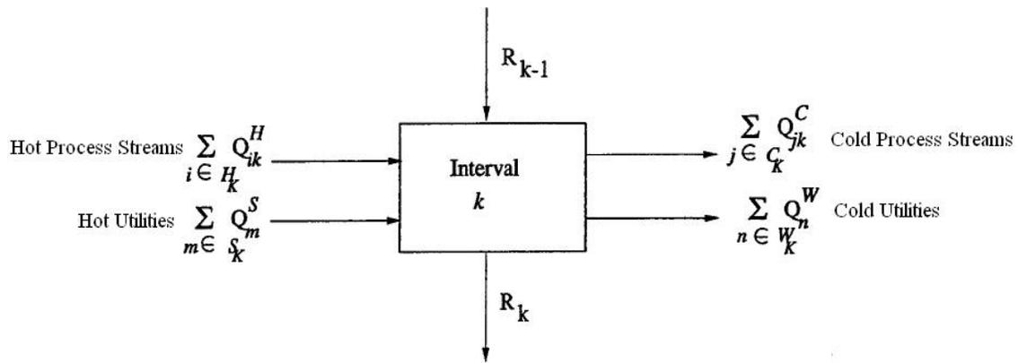
Figure 2: Heat flow pattern for a given temperature interval.
