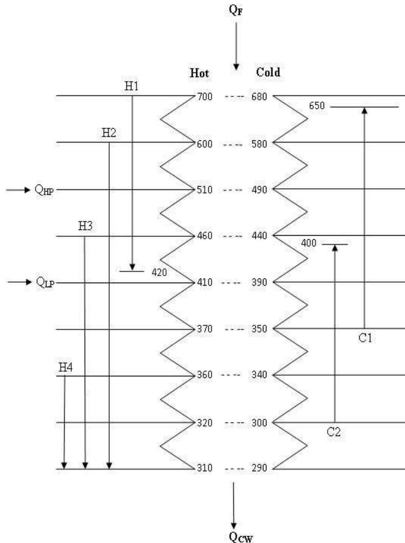
**Figure 1:** Temperature interval diagram for minimum utility cost problem.
