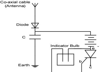
**Figure** 4: Ambient energy generation using co-axial cable – investigating the electret effect The results of this investigation are presented in Table 3 based on using co-axial cable with outer plastic sheath present.
