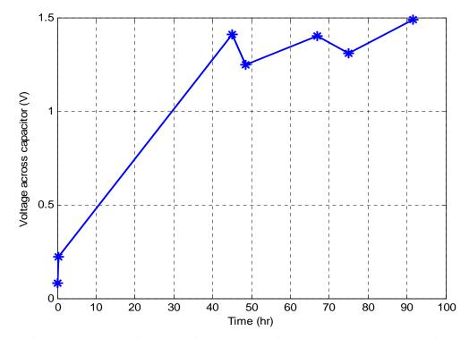
Figure 3: Plot of voltage across capacitor against time for the modified ambient energy transducer without electret effect.
