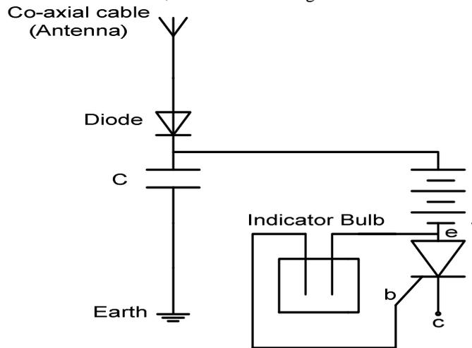
**Figure 4:** Ambient energy generation using co-axial cable – investigating the electret effect
