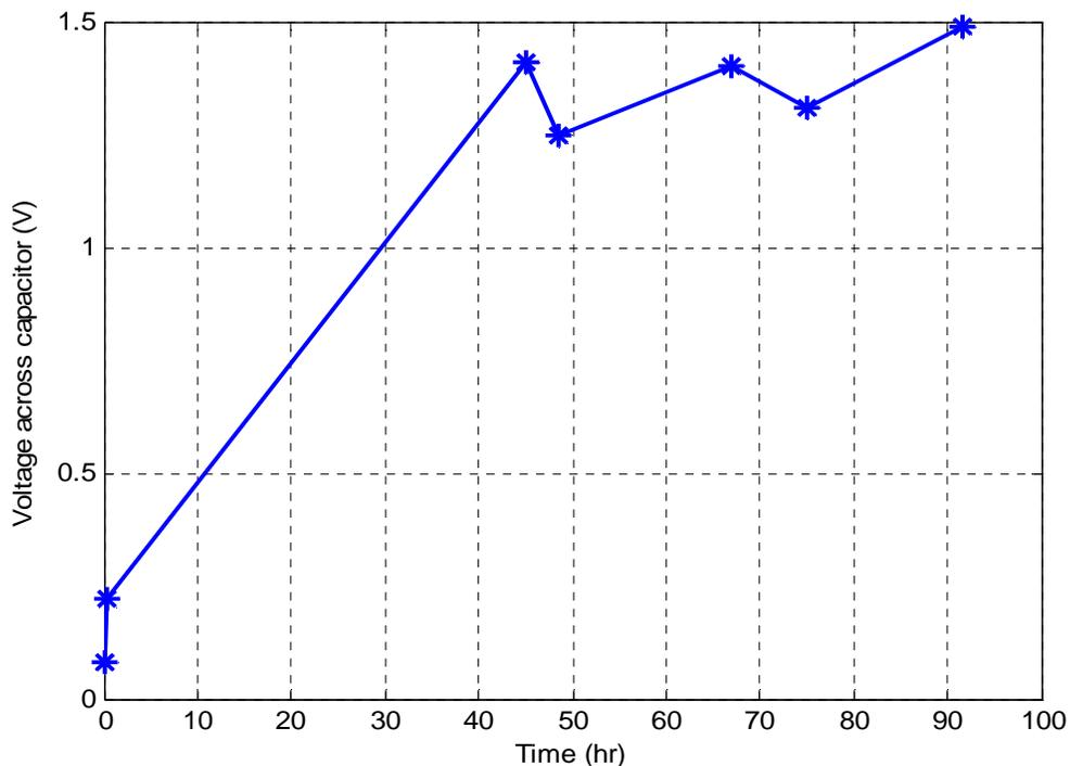
**Figure 3:** Plot of voltage across capacitor against time for the modified ambient energy transducer without electret effect.
