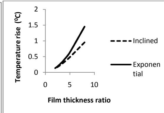
Figure 5: Temperature rise as a function of film thickness ratio for  $p_{inlet} = 101\text{Kpa}$
