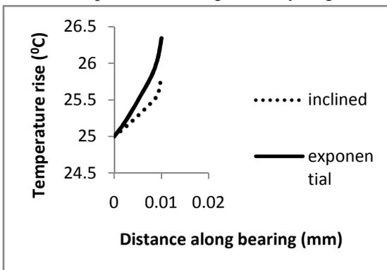
Figure 4: Temperature profile for inclined and exponential slider bearings for  $p_{inlet} = 101\text{Kpa}$
