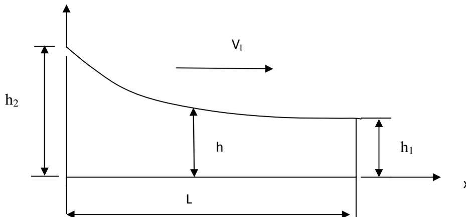
Figure 2: Schematic drawing of exponential film shape slider bearing
