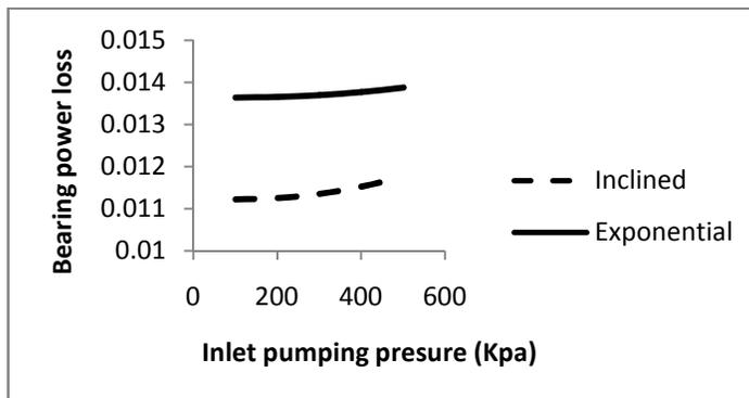
Figure 6: Bearing power loss as a function of inlet pumping pressure ( $r = 8$ )
