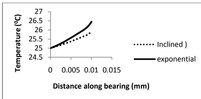
**Figure 3:** Temperature profile for inclined and exponential slider bearings for  $p_{inlet} = 101 \text{Kpa}$
