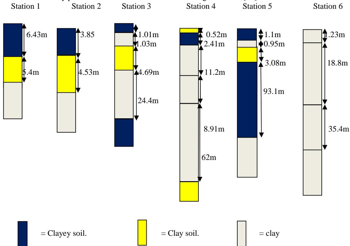
Figure 5.7: clay positions and thicknesses for stations 1-6 [20]
