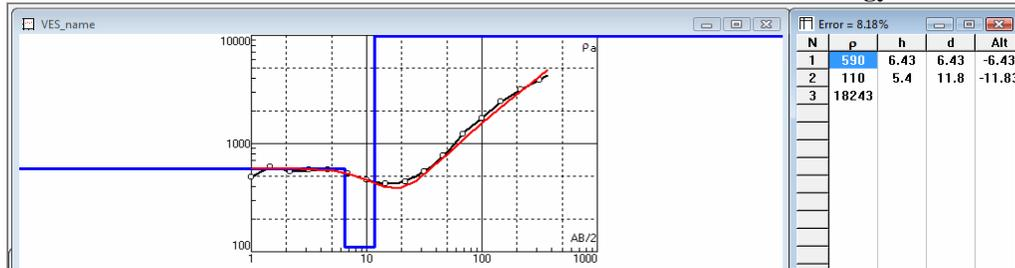
**Fig 5.1: Iterated sounding curves for station 1**
