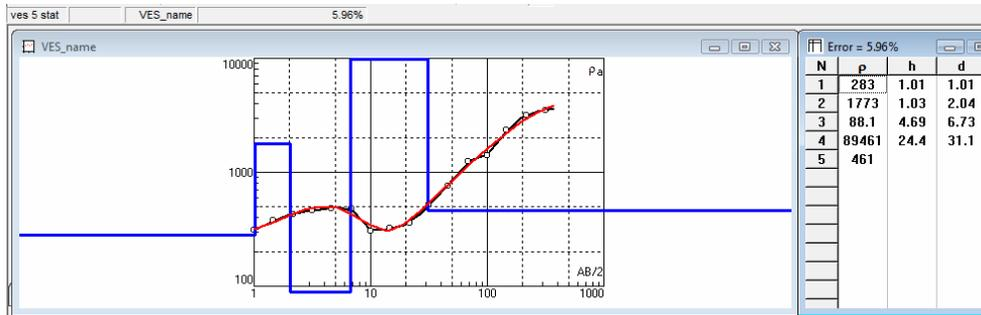
Fig 5.3: Iterated sounding curves for station 3
