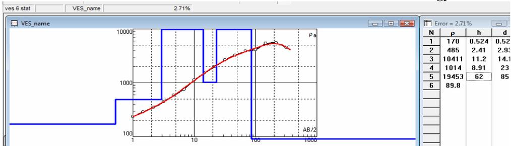
Figure 5.5: iterated sounding curve for station 5
