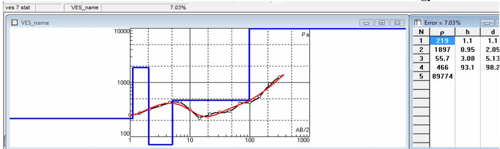
Fig 5.4 : Iterated sounding curves for station 4
