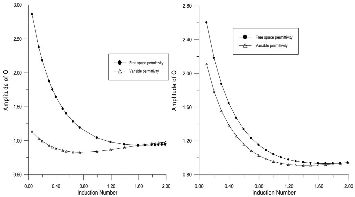
**Figure 11.** Plot of the Amplitude of Q versus Induction Number ( $k = 0.1$ )
