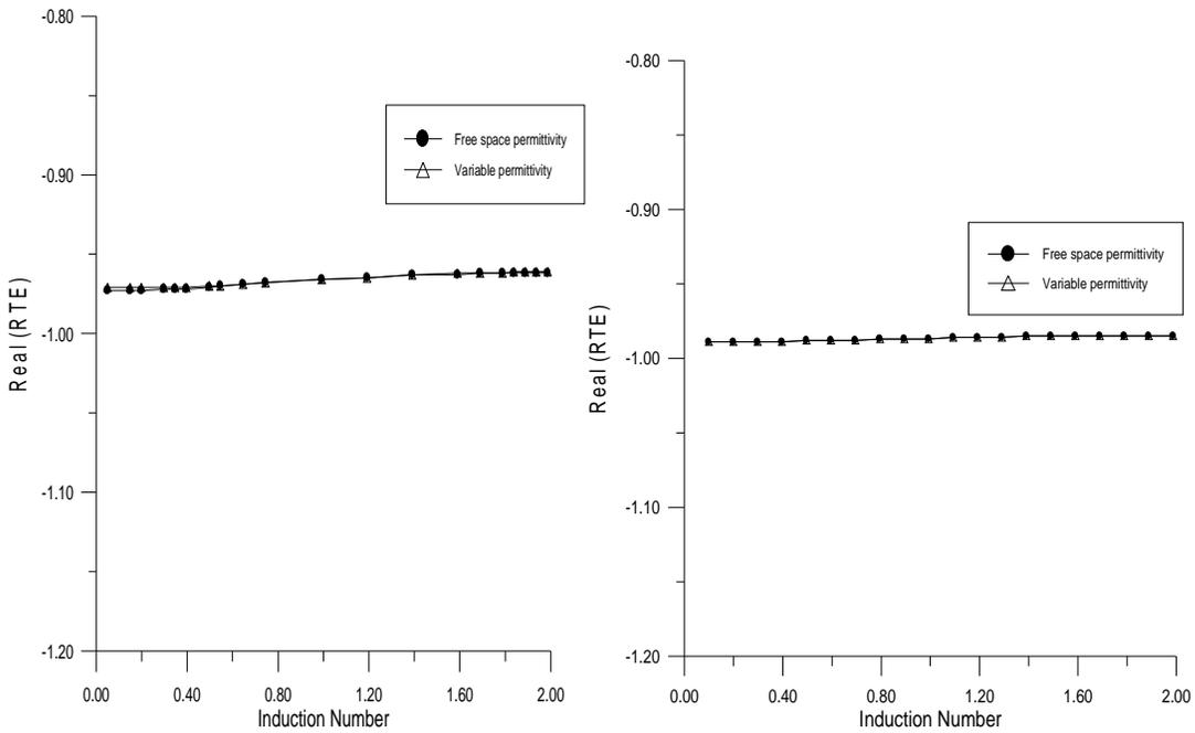
**Figure 4.** Plots of the Reflection coefficient (TM & TE mode) versus Induction ( $k = 2$ )
