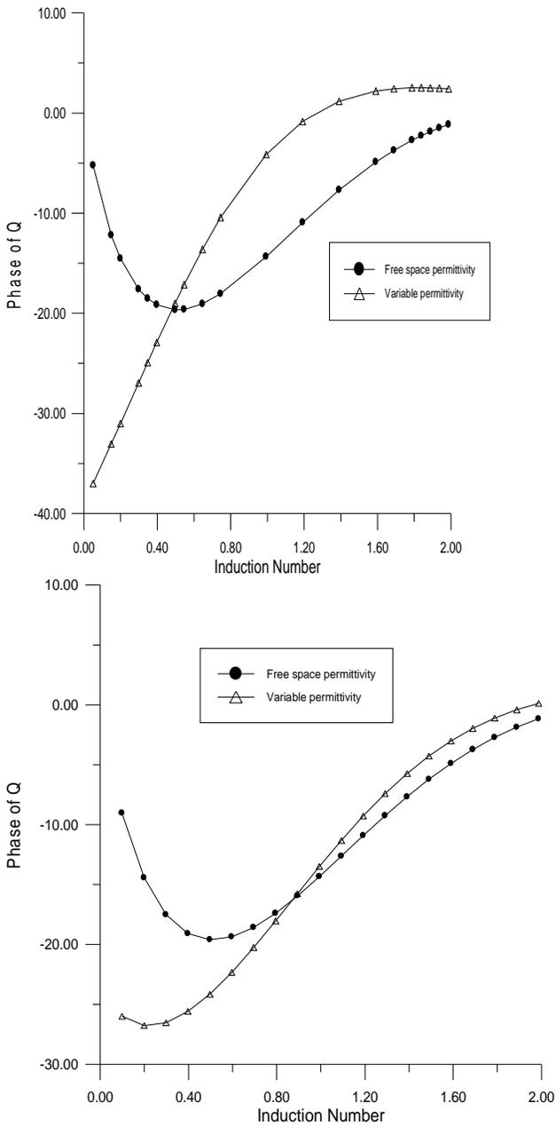
**Figure 12.** Plot of the Phase of Q versus Induction Number ( $k = 0.1$ )
