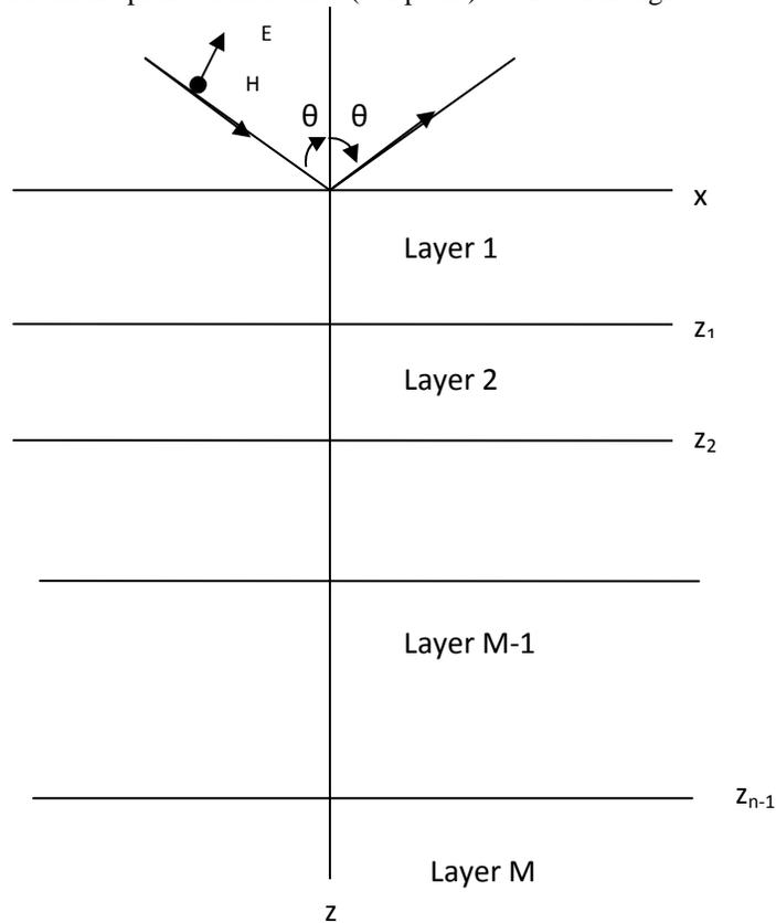
**Figure 2.1** Coordinate system for the stratified medium of  $M$ -layers.
