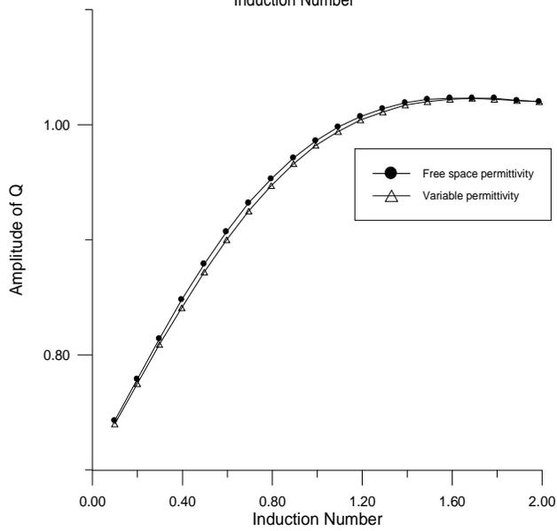
**Figure 2.** Plot of the Amplitude of Q versus Induction Number ( $k = 2$ )
