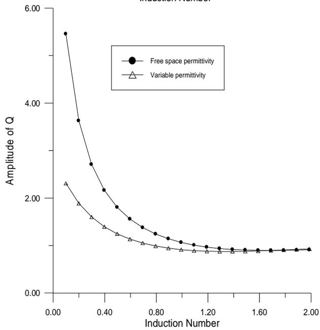
**Figure 14.** Plots of the Amplitude of Q versus Induction Number ( $k = 0.01$ )
