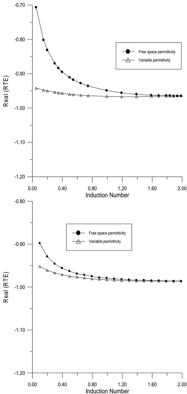
**Figure 16.** Plots of the Reflection coefficient (TM & TE mode) versus Induction ( $k = 0.01$ )
