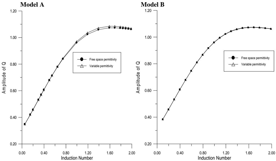
**Figure 5.** Plot of the Amplitude of Q versus Induction Number ( $k = 10$ )
