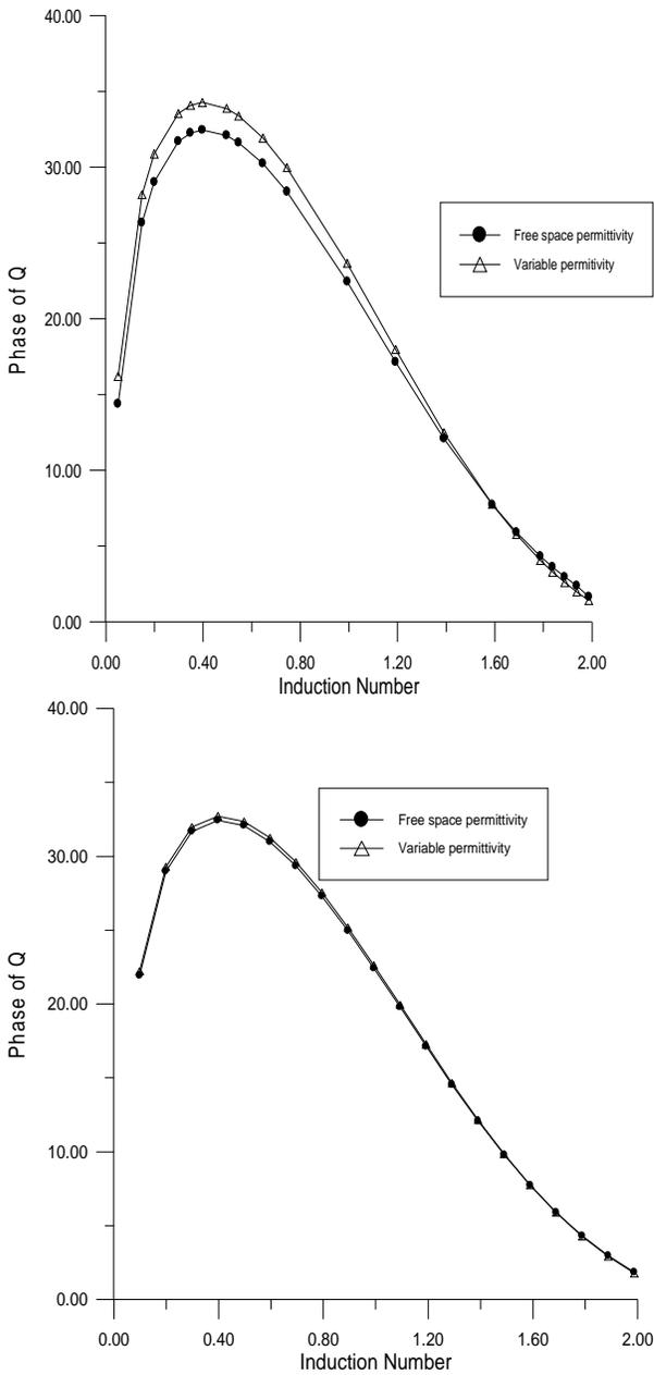
**Figure 9.** Plot of the Phase of Q versus Induction Number ( $k = 100$ )
