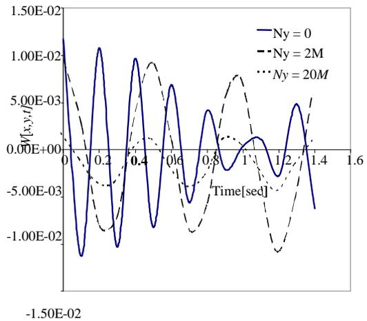
**Figure 7.10:** Deflection profile of simply-clamped rectangular plate traversed by moving mass for fixed  $Ro=10$ ,  $N_x=2M$ ,  $K=2M$  for various values of  $N_y$
