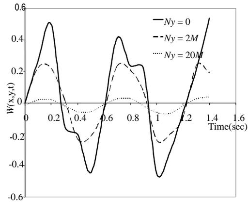
**Figure 7.4:** Deflection Profile of Simply-Supported Rectangular Plate Traversed by Moving Mass for fixed  $R_0=10, N_x=2M, K=2M$  for various values of  $N_y$
