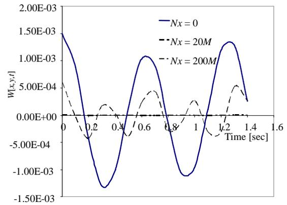
**Figure 7.9:** Deflection profile of simply-clamped rectangular plate traversed by Moving Mass for fixed  $Ro=10$ ,  $N_y=2.5$ ,  $K=2M$  for various values of  $N_x$
