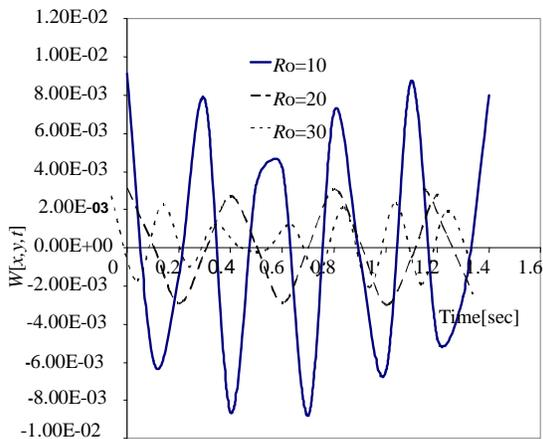
**Figure 7.7:** Deflection profile of simply-clamped rectangular plate traversed by moving mass for fixed  $N_x=2M$ ,  $N_y=2.5M$ ,  $K=2M$  for various values of  $Ro$
