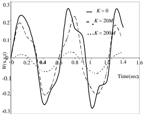
**Figure 7.2:** Deflection profile of simply-supported rectangular plate traversed by moving mass for fixed  $N_x = 2M$ ,  $N_y = 2.5M$ , for various value of  $K$
