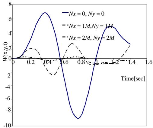
**Figure 7.5:** Deflection profile of simply-supported rectangular plate traversed by moving Mass for fixed  $Ro=10$ ,  $K=2M$  when values of  $N_x$  and  $N_y$  are increase simultaneously
