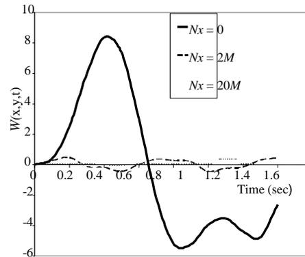
**Figure 7.3:** Deflection profile of simply-supported rectangular plate traversed by moving mass for fixed  $R_0 = 10$ ,  $N_x = 2.5M$ ,  $K = 2M$  for various values of  $N_x$
