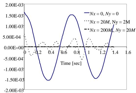
**Figure 7.11:** Deflection profile of simple-clamped rectangular plate traversed by moving mass for fixed  $Ro=10$  and  $K=2M$  when values of  $Nx$  and  $Ny$  are increase simultaneously.
