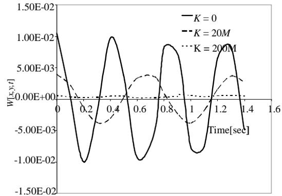
**Figure 7.8:** Deflection profile of simple-clamped rectangular plate traversed by moving mass for fixed  $Ro=10$ ,  $N_x=2M$ ,  $N_y=2.5$  for various values of  $K$ .
