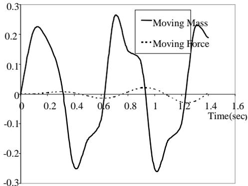
**Figure 7.6:** Comparison of the deflection of moving force and moving mass cases for simple supported rectangular plate for fixed  $Ro=10$ ,  $K=2M$ ,  $N_x=2M$  and  $N_y=2.5M$
