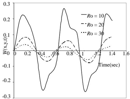
**Figure 7.1:** Deflection profile of simply-supported rectangular plate traversed by moving mass for fixed  $N_x = 2M$ ,  $N_y = 2.5M$ ,  $K = 2M$  for various values of  $R_0$ .
