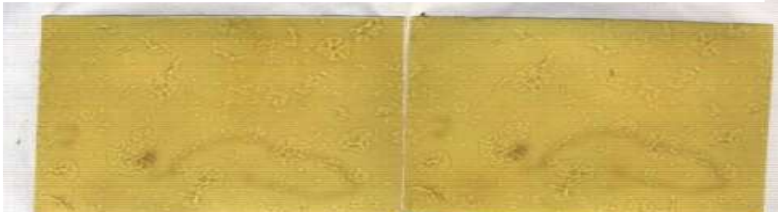
Figure 12: Electron micrograph of CdS thin film deposited at 300K
