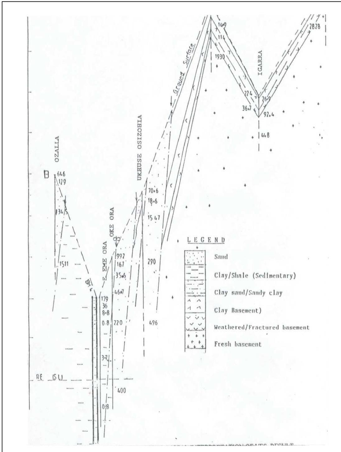
**Figure 3:** Cross section B-B showing geological interpretation of VES result correlated with borehole records.
