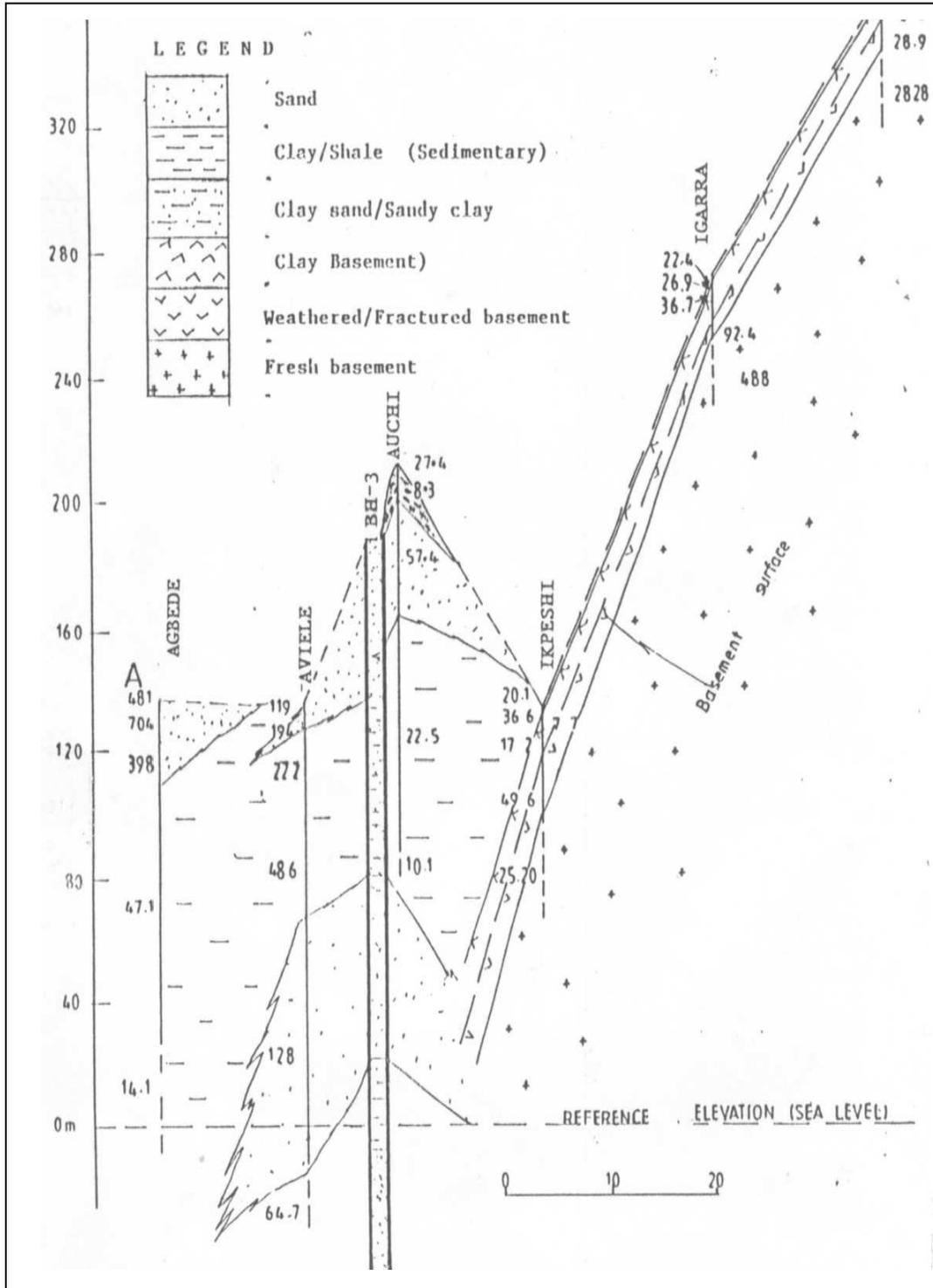
**Figure 4:** Cross section B-B showing geological interpretation of VES result correlated with borehole records.
