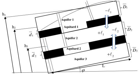
Figure 1: A cross-section of a sloping three-aquifer system of hillslope length, L at an angle  $\varphi$  to the horizontal in aquifer 1, aquifer 2 and aquifer 3.
