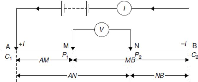
Figure 2: Generalized form of electrode configuration in resistivity surveys.
