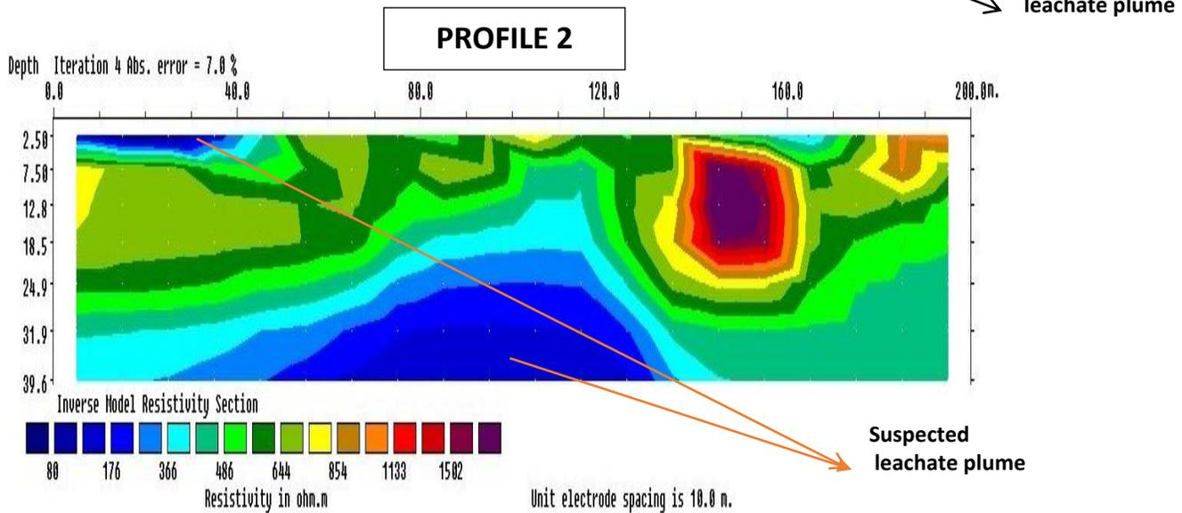
**Figure 4: Inverted 2D resistivity pseudo-sections of profile two**
