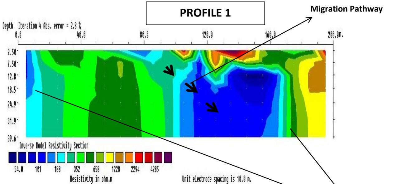
**Figure 3: Inverted 2D resistivity pseudo-sections of profile one**
