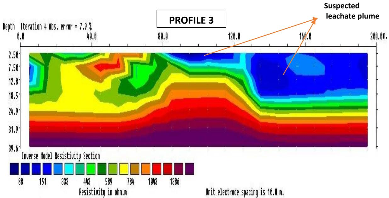
Figure 5: Inverted 2D resistivity pseudo-sections of profile three
