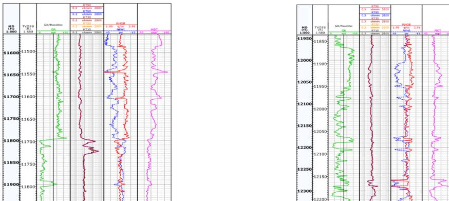
Figure 3.9: Wire line log for Well X containing Gamma ray log, resistivity log, and neutron density log (continuation).
