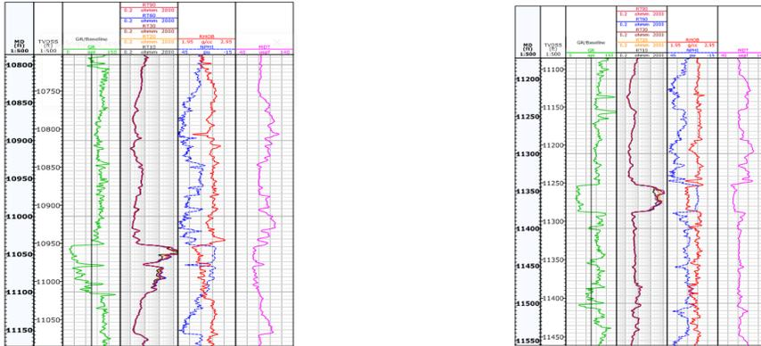
Figure 3.8: Wire line log for Well X containing Gamma ray log, resistivity log, and neutron density log (continuation).
