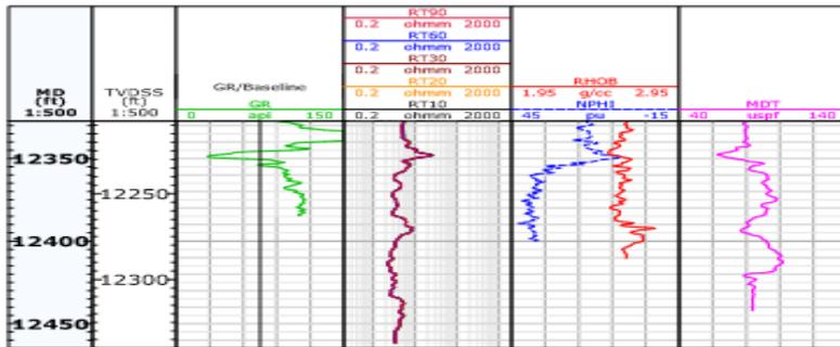
Figure 3.10: Wire line log for Well X containing Gamma ray log, resistivity log, and neutron density log (continuation).
