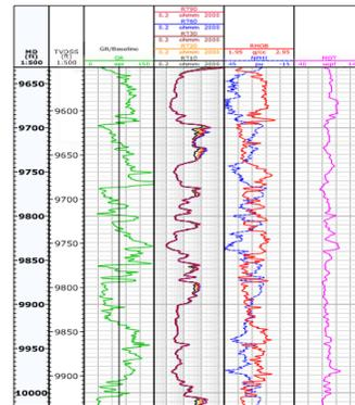
Figure 3.6: Wire line log for Well X containing Gamma ray log, resistivity log, and neutron density log (continuation).
