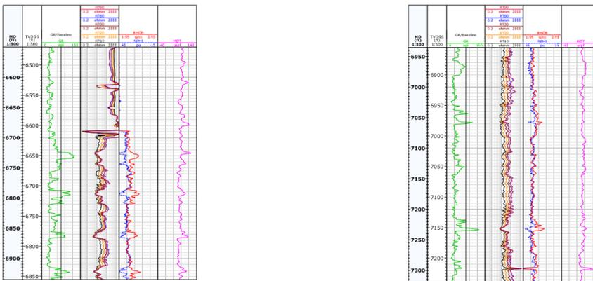
Figure 3.2: Wire line log for Well X containing Gamma ray log, resistivity log, and neutron density log.
