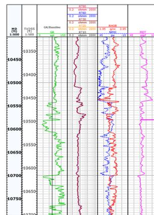
Figure 3.7: Wire line log for Well X containing Gamma ray log, resistivity log, and neutron density log (continuation).
