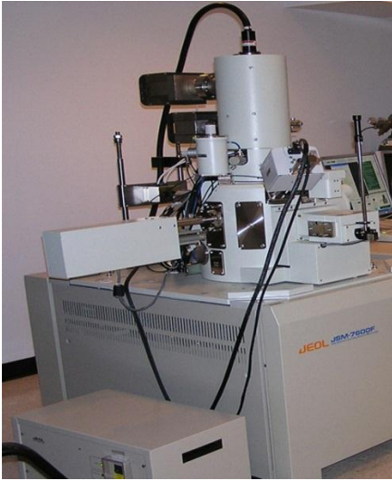
Figure 2.2: Photograph of a Scanning Electron Microscope (SEM)
