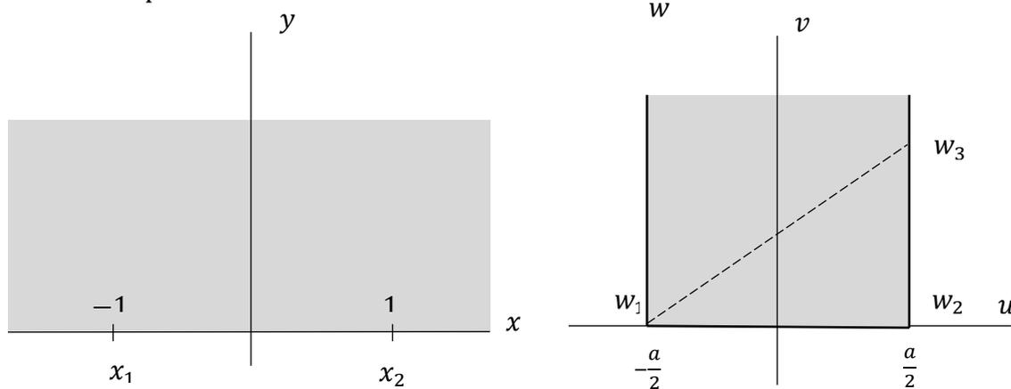
Figure 1(a): One-to-One Mapping of the Half Plane  $\text{Im } z \geq 0$  in the  $z$  plane Onto the Semi-Infinite Strip in the  $w$  plane
