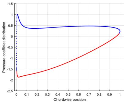
**Figure 3(b): Pressure Coefficient Distribution Against Chordwise Position on the Cambered Joukowski Airfoil in figure 3(a) at  $10^\circ$  Flow Angle of Attack (Blue Line- $c_p$  on Lower Surface, Red Line- $c_p$  on Upper Surface)**
