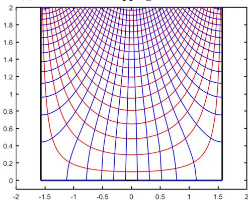
Figure 1(b): Equipotential (Blue) and Streamlines (Red) of flow in the Interior of a Semi-Infinite Strip the  $w$  plane.
