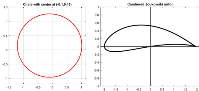
**Figure 3(a): Circle with Centre at  $z = -0.1 + 0.15i$  and Corresponding Mapped Cambered Joukowski Airfoil for the Case  $c = 1$  in the Joukowski Transformation**
