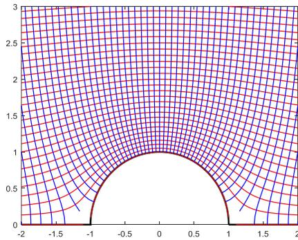
**Figure 2(b): Equipotential Lines (Blue) and Streamlines (Red) of flow in the Domain of the First Diagram of figure 2(a).**
