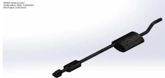
Figure 2: Mesh Visualization of the Exhaust Model
