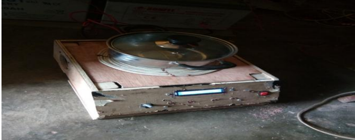
Appendix B: Testing with a regular cooking pot for heating effects
