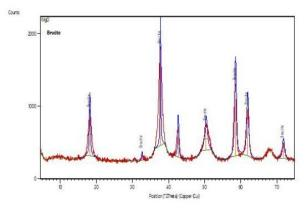
Figure 2: XRD of MgO Nanoparticles **XRF**
