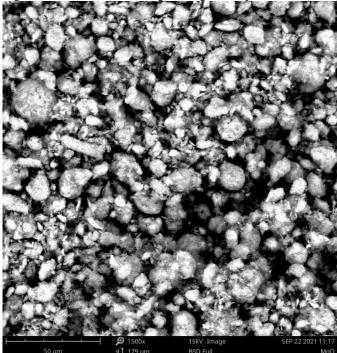
Figure 1: SEM of MgO **XRD**
