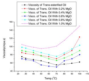
Figure 3: Viscosity Versus Temperature of Rapeseed Oil
