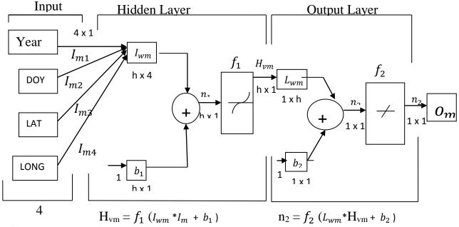
Figure 2: Neural Network Training Structure from Input to Output
