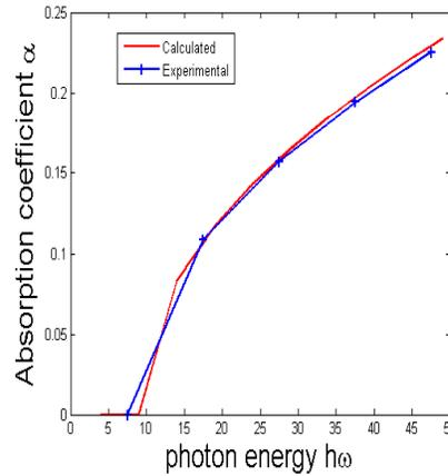
Figure 18: Calculated and Experimental Absorption Coeff. Vs Photon energy.
