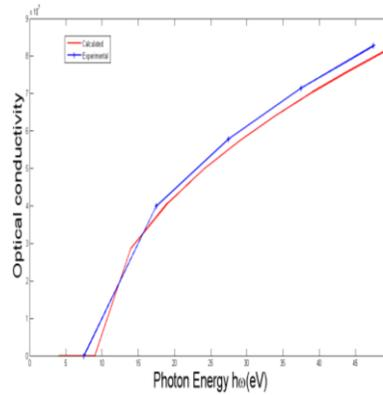
Figure 20: Calculated and Experimental Optical Conductivity Vs Photon energy
