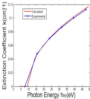
Figure 19: Calculated and Experimental Extinction Coeff. Vs Photon energy
