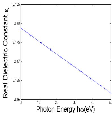
Figure 15: Real Dielectric Constant Vs Photon energy
