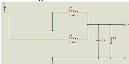
Fig. 5 Equivalent circuit of IBC in mode 3
