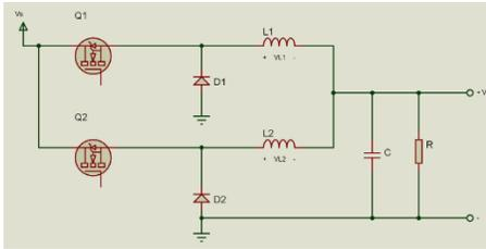
Fig. 2 Circuit diagram of a two-phase interleaved buck converter
