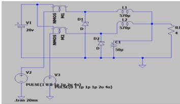
Fig. 7 LTSpice circuit diagram for interleaved Buck converter
