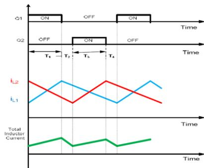
Fig. 6 Inductor current waveform
