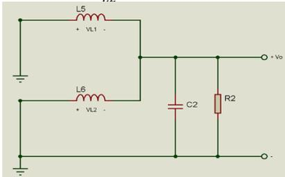
Fig. 4 Equivalent circuit of IBC in mode 2
