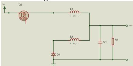
Fig. 3 Equivalent circuit of IBC in mode 1
