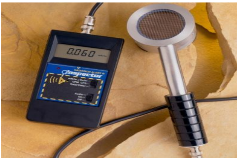
Figure 1. The Handheld Radiation Detector (Radiation Alert Inspector EXP + )
